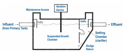
1. An aerator requires the use of a motor to bring air into the system and create good bacteria known as aerobic bacteria. These bacteria break down sewage, producing a clean effluent. If you have an aerator, check often to ensure that the motor is running properly. You should be able to hear your aerator when standing beside it, and you can also feel vibrations if you put your hand on it.
